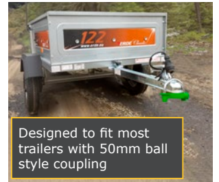
Case hardened Solid Steel 12.6mm diameter top U bar, with 11 locking positions
